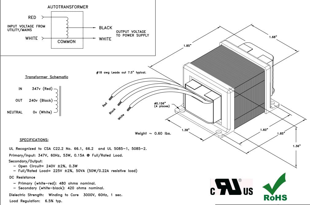
Efficiency: 94% typ. @ 347Vin, 50VA load.
