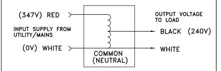
Note: "FB" version has an internal auto reset 110°C thermal protector in series with the "RED" input lead.
